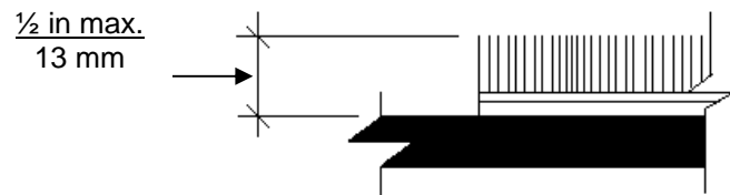
Fig. 8(f) Carpet Pile Thickness
